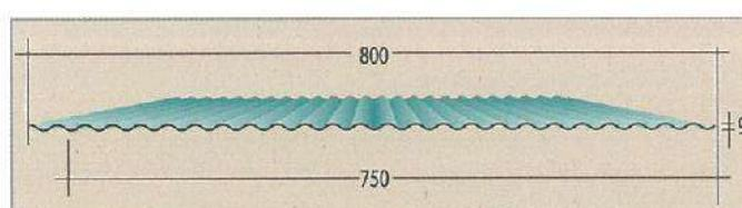
**D 750**      Thickness: 20-30 Bj.L.S      Minimum Length: 1,50 m      Maximum Length: 3,65 m
