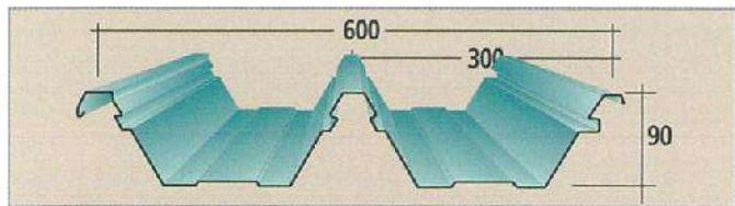
**BL 600**    Thickness: 45-80 Bj.L.S    Minimum Length: 1,5 m    Maximum Length: 12 m
