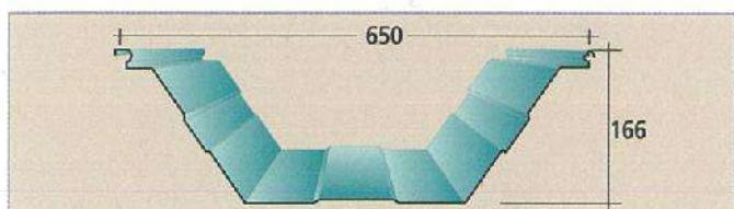
**SF 650**    Thickness: 45-100 Bj.L.S    Minimum Length: 1,5 m    Maximum Length: 12 m
