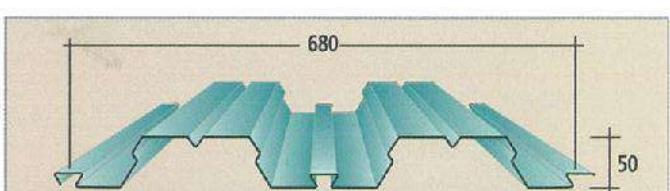
**COMPODECK**    Thickness: 70-100 Bj.L.S    Minimum Length: 1,00 m    Maximum Length: 12 m
