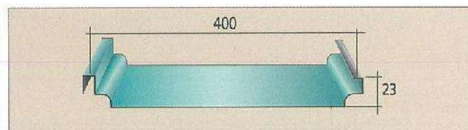
**SF 400**      Thickness: 35 - 50 Bj.L.S      Minimum Length: 1,00 m      Maximum Length: 12 m
