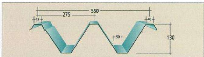
**GP 550**    Thickness: 45-80 Bj.L.S    Minimum Length: 1,5 m    Maximum Length: 12 m
